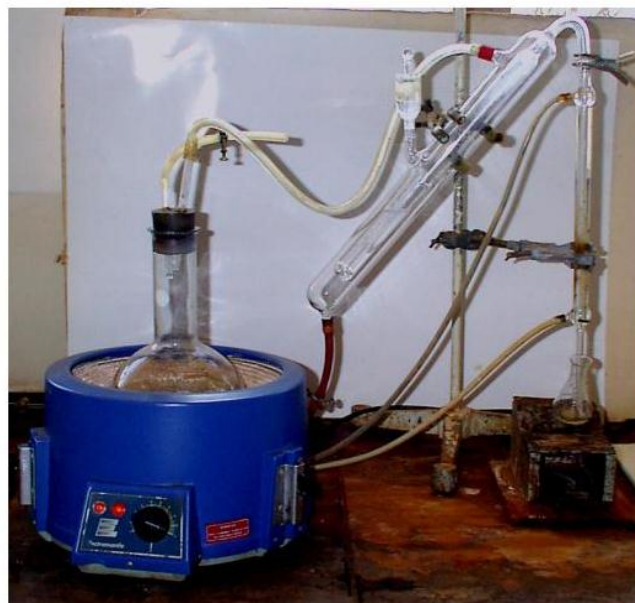
Figure 9.1. Nitrogen steam distillation apparatus
